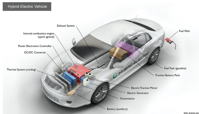
Figure 3: Key Components of a Hybrid Electric Car
