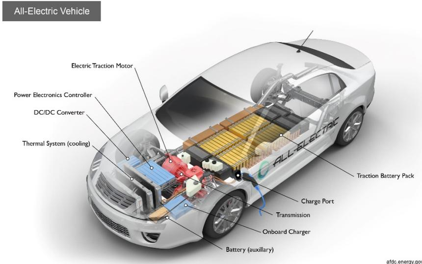
Figure 4: Key Components of an Electric Vehicle
